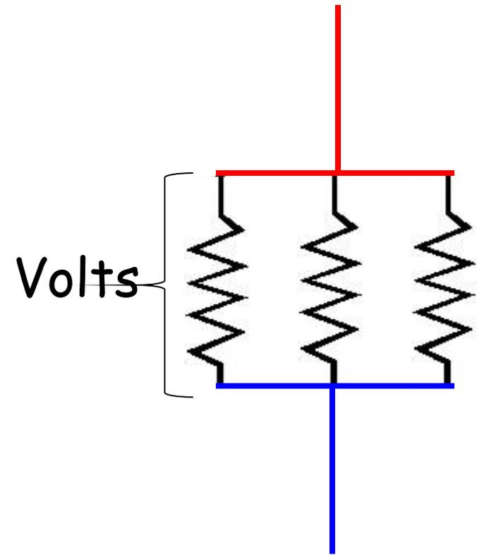
$$\frac{1}{R_{total}} = \frac{1}{R_1} + \frac{1}{R_2} + \frac{1}{R_3}$$
