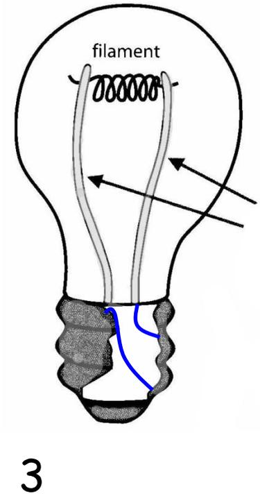
Where do these two wires connect to the base of the light bulb? Which bulb is wired correctly?
