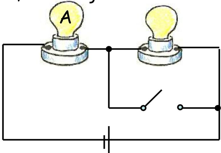
The circuit below consists of two identical light bulbs burning with equal brightness and a single 12V battery. When the switch is closed, the brightness of bulb A...
