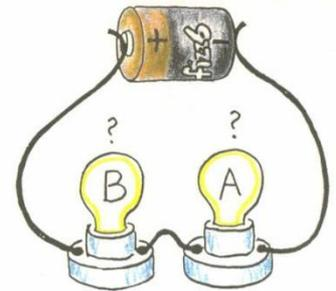
The bulbs are connected in series, so the same current passes through both of them. Different brightnesses indicate different filament resistances. Bulb A is NOT brighter because it is "first in line" for the current of the battery! After all, electrons deliver the energy, and they flow from negative to positive --- in the opposite direction!
