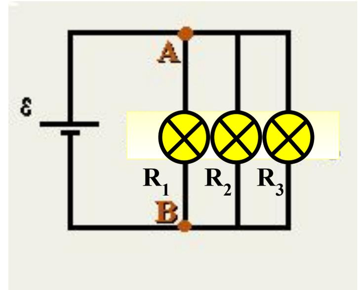
Given:  $R_1=1\Omega$ ;  $R_2=2\Omega$ ;  $R_3=3\Omega$ . Rank the bulbs according to their relative brightness
