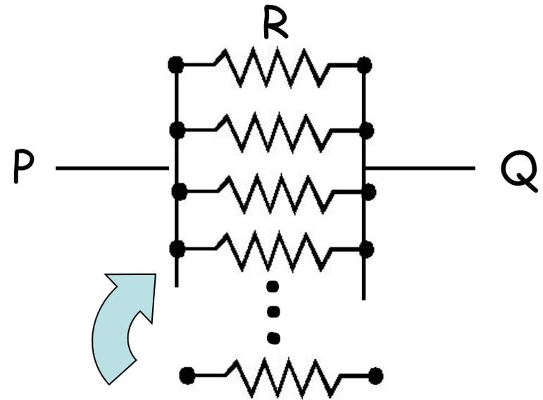
As more identical resistors  $R$  are added to the parallel circuit shown, the total resistance between points  $P$  and  $Q$  ...
