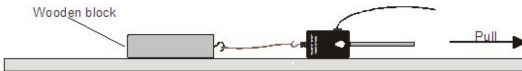
2. An easy way to do this with logger pro is to click the green arrow to collect data and GENTLY pull the sensor horizontally 4 or 5 times so that the graph produces 4 or 5 similar force peaks on the graph. Once the run is done, you can use the EXAMINE function to figure out the maximum force for each peak which = the static friction force that needed to be overcome to move the block. Don't forget to zero the sensor before starting.
