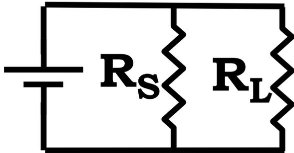
**Which resistor has a larger voltage drop, the larger resistor ( $R_L$ ) or the small resistor ( $R_S$ )?**
