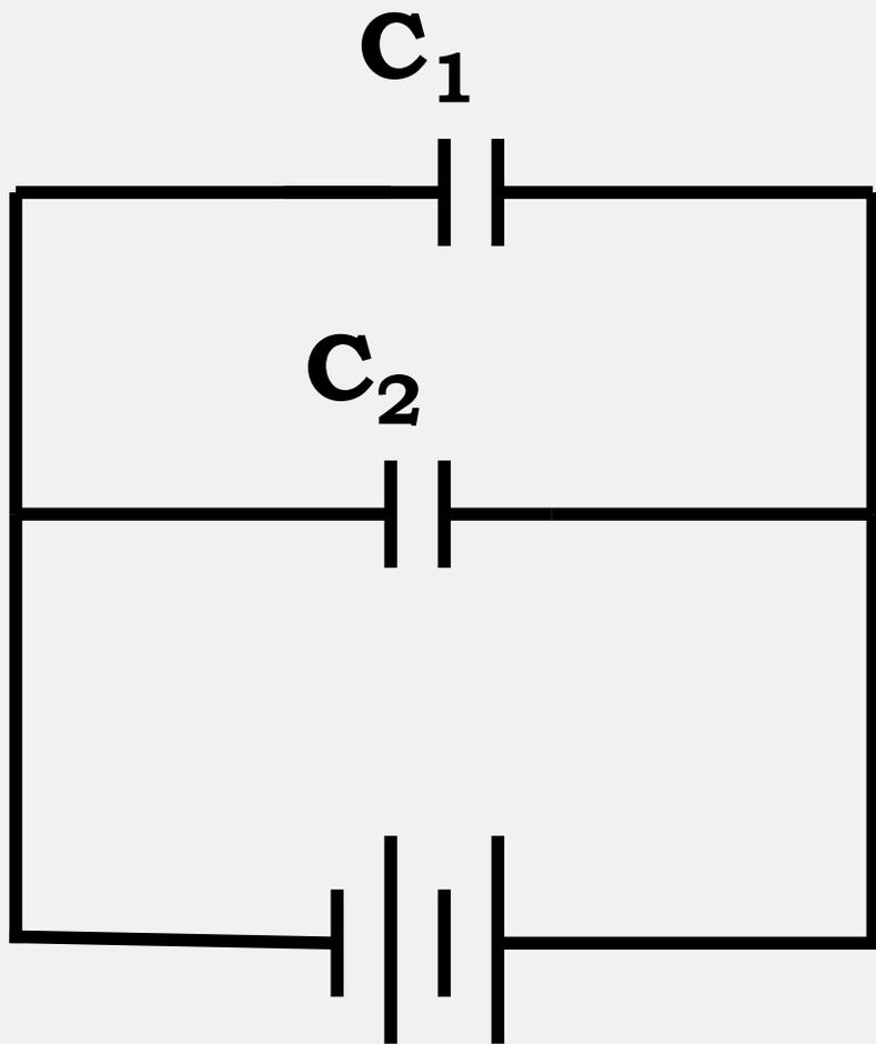
If  $C_1 < C_2$ , which capacitor has the largest voltage drop across it?
