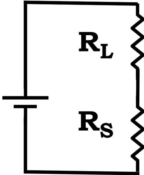
**Which resistor has more current flowing through it, the larger resistor ( $R_L$ ) or the small resistor ( $R_S$ )?**
