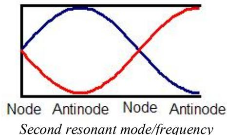
*Open Pipe:* Just like with a closed pipe an open pipe can support a standing wave. The boundary conditions are that there must be antinodes at both ends of the pipe.
