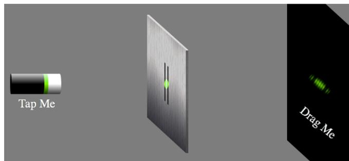
The middle section represents the front view of the screen. This view allows you to see the actual interference pattern consisting of bright and dark bands. These bands are the result of the wave interference of the waves for the waves diffracting through the two slits. The cm-ruler can be used to measure the distance between bright bands on the interference pattern.
