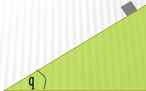
Draw a free-body diagram for a block accelerating down a ramp.
