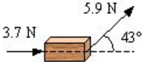
Resolve into components, Add the forces, then find  $F_{\text{net}} = ma$ .
