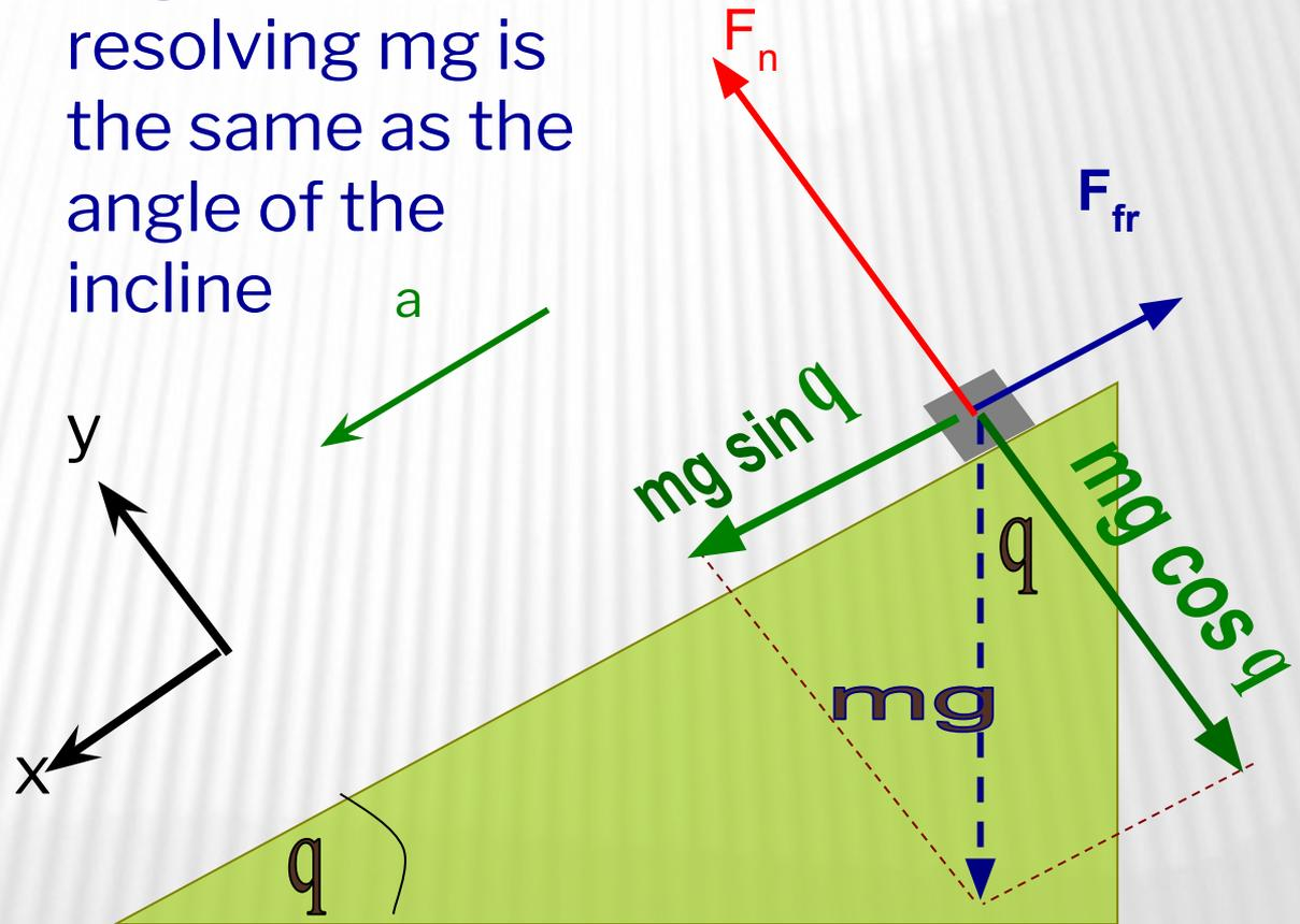
Resolve vector  $mg$  into two components. Now instead of three forces, we have four forces
