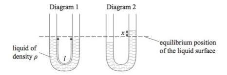
The pressure on the liquid in one side of the tube is increased so that the liquid is displaced as shown in diagram 2. When the pressure is suddenly released the liquid oscillates. The damping of the oscillations is small.
