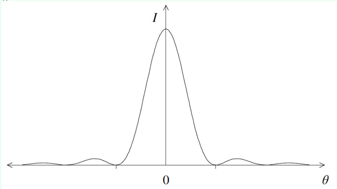
overall correct shape with central maxima at  $\theta=0$ ; { *only one secondary maximum required each side of  $\theta=0$*  }
