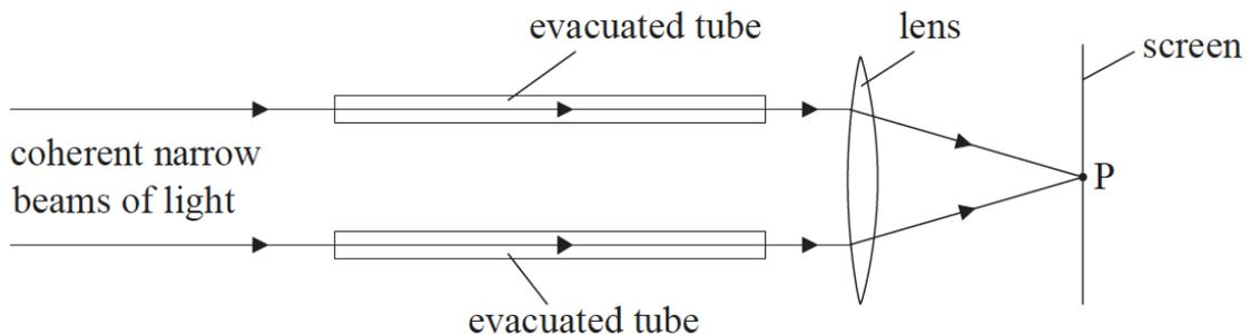
The two coherent narrow beams are brought to a focus at point P on a screen.
